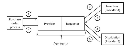
Figure 1.1: Example of a system with 6 XML schemas
